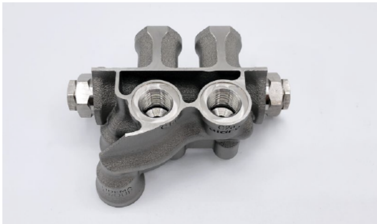
Fig. 2 A hydraulic block for a marine application, designed by Aidro and additively manufactured in 316L stainless steel for Fidema Group. The use of AM allowed a reduction in the number of hydraulic fittings that regularly leaked hydraulic fluid, a reduction in the overall dimensions, and the creation of a design optimised for the narrow space available. The arrangement of the cylinder control ports is customised according to the body orientation, not 'in-line', but with 90° exits [Courtesy Aidro]
