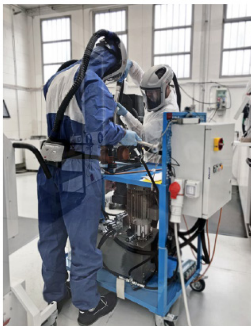
Fig. 5 Manual post-build operations include separation of parts from the build plate and support removal (Courtesy Aidro)
