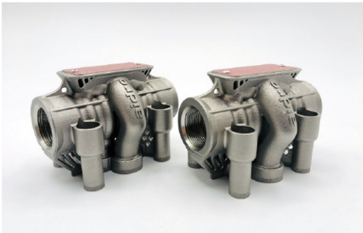
Fig. 7 Small AMES valves for hydraulic systems. AMES are CETOP directional control valves, here additively manufactured in 316L stainless steel and designed to work at 350 bar. These AM valves underwent high-pressure testing up to 1,400 bar (Courtesy Aidro)
