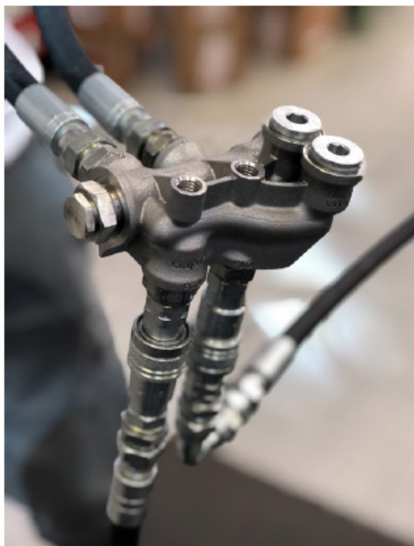
Fig. 3 Testing of the hydraulic block shown in Fig. 2 which, thanks to the optimisation of the design, enabled a weight reduction from 3.8 kg of the conventional part to 0.63 kg for the AM part (Courtesy Aidro)
