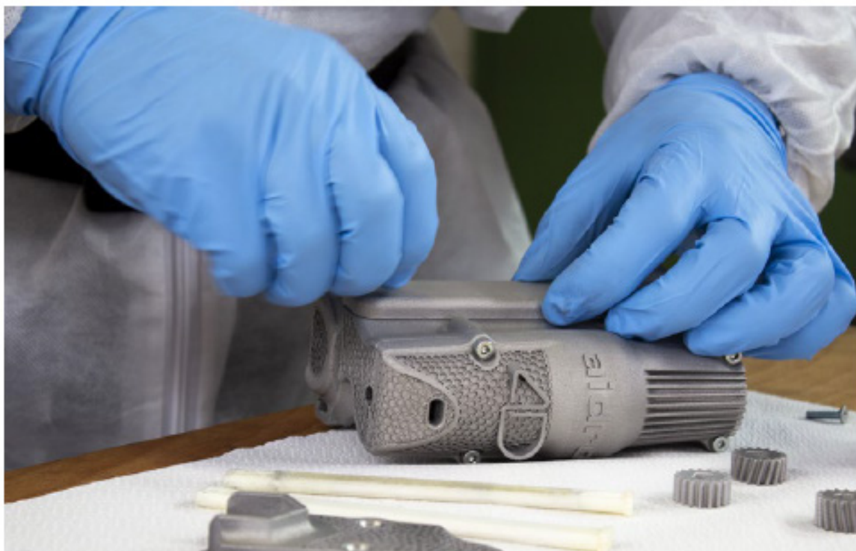
Fig. 8 An accessible aeronautic system that allows pilots who have only one hand to fly safely and easily. The AM flight control parts shown, manufactured by Aidro, are used in the Servofly system ( www.servofly.it/en/ ) (Courtesy Aidro)
