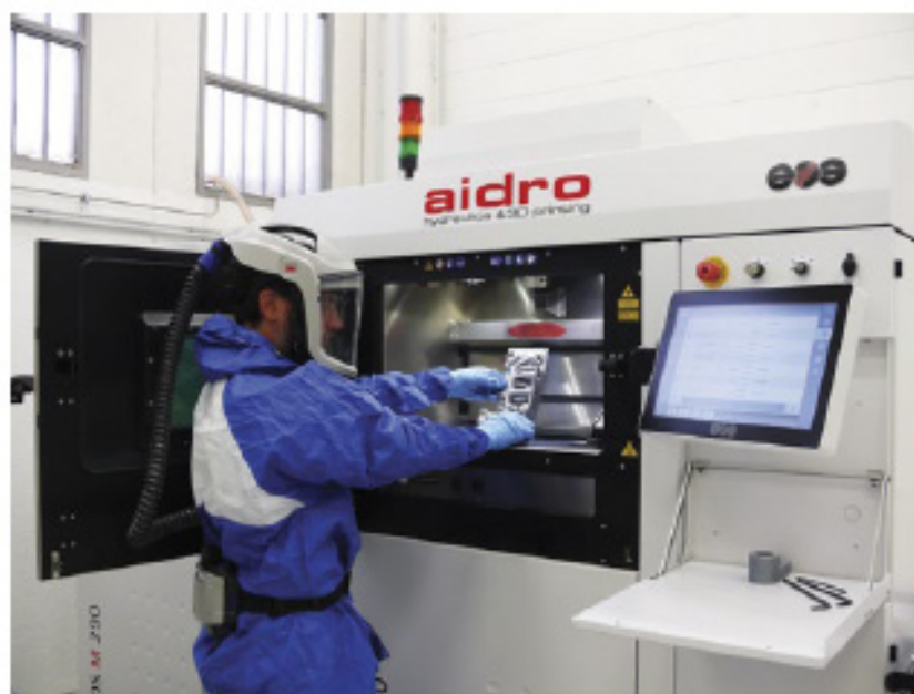
Fig. 4 An EOS M 290 PBF-LB machine at Aidro (Courtesy Aidro)
