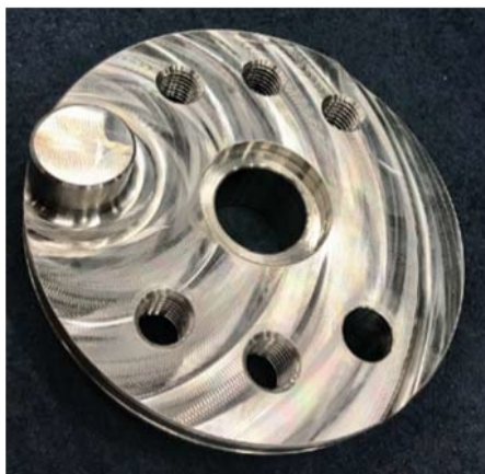
The crank disk 3D printed by Aidro with EOS M290 and machined by Kongsberg.
