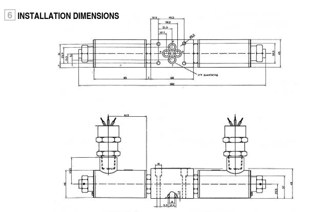
All valves HD3-\* conform with ISO and CETOP specifications for mounting surface dimensions (see also front page) and for valves height. When assembled to its mounting plate valve HD3-\* must be fastened with 4 bolts M5 X 45 mm (or M5 x \*\* according to the number of modules) tightened at 8 Nm torque. Leakage between valve and mounting surface is prevented by the positive compression on their seats of 4 seals of QUAD/O Ring type 9,25x1,68x1,68.
