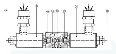
The spool 12 shifts into the valve body 11 subject to the action of springs 13 and solenoids 2. Spool 12, depending from its shape and its position in the valve body, opens and/ or closes passages between P, A, B and T ports, thus controlling the direction of the hydraulic flow.
