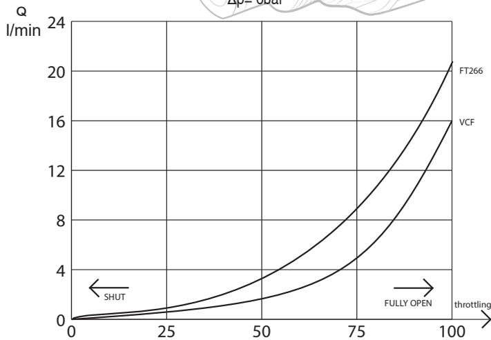
Typical Q curves a different throttling sections and fixed  $\Delta p = 6 \text{ bar}$  for valves FT266/VCF. Standard configuration with mineral oil at 42cSt and 50° C.
