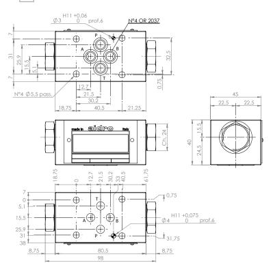
All stackable valves AM3 -\* conform with ISO and CETOP specifications for mounting surface dimensions. Valves height 40 mm. Leakage between valve and mounting surface is prevented by the positive compression on their seats of 4 seals of OR type. All valves have on their "mounting" surface a  $\varpi$  4 mm cylindrical hole and have on their "seals" surface a  $\varpi$  3 mm cylindrical hole, conform with ISO and CETOP norms.
