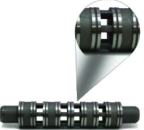
Because it is not bound by conventional manufacturing techniques, 3D printing can produce components with unconventional shapes. The benefits can be realized in components such as this valve spool with square ports for greater flow capacity than round ports of the same width. (Image courtesy of Aidro SrL)
