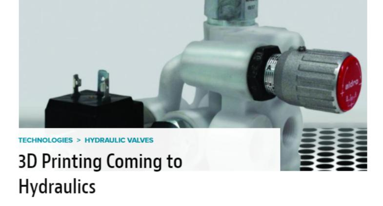
The challenges of high pressure have kept metal 3D printing from gaining widespread application in hydraulics technology, but we may begin seeing 3D-printed components in specialized applications.
