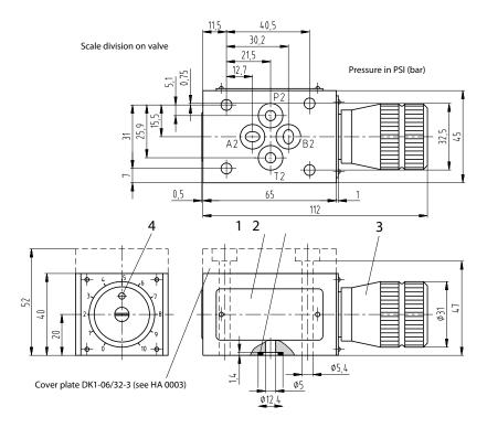
All stackable valves AM3-Q3- \* conform with ISO and CETOP specifications for mounting surface dimensions and for valves height 40 mm. Leakage between valve and mounting surface is prevented by the positive compression on their seats of 4 seals type OR 2037.
