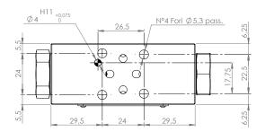
All stackable valves AM2-CP-\* conform with ISO and CETOP specifications for mounting surface dimensions (see also front page). Valves height 35 mm. Leakage between valve and mounting surface is prevented by the positive compression on their seats of 4 seals of OR type. All valves have on their "mounting" surface a ø 4 mm cylindrical hole and have on their "seals" surface a ø 3 mm cylindrical hole, conform with ISO and CETOP norms.
